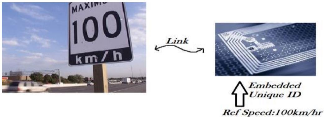
Figure 3. Tag connected to speed limit boards on the side of the road
